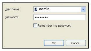
**3.** Enter **admin** for the WiFi modem router user name and **password** for the WiFi modem router password, both in lowercase letters.
